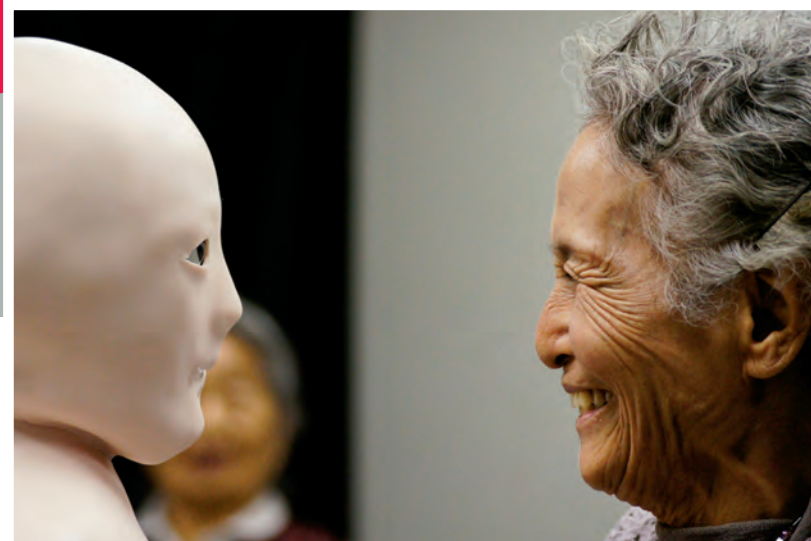
This model, called the Telenoid, is meant to be a generic android that anyone can use to transmit their presence somewhere else. Users young or old, male or female, could speak through the Telenoid just like Ishiguro with his Geminoid.
